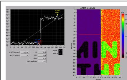
Fig.4: Thickness profile (in nm, left) along red line in the thickness map right, recorded within 1 minute, 4 μm lateral resolution according to the sample area shown in fig.1 and 3.
