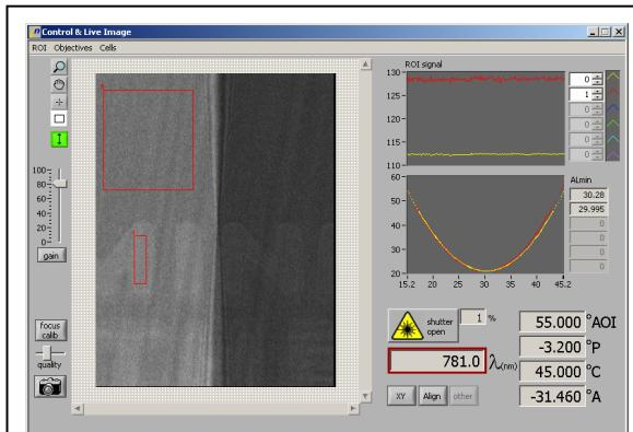
Fig. 1: "Control & Live Image" with Regions Of Interest (boxes no. 0 and 1 in the ellipsometric contrast live image on the left)
