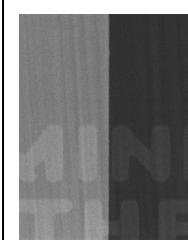
Fig.3: Ellipsometric contrast image focussed by objective scan, 55° angle of incidence, 781 nm wavelength, 350 μm x 450 μm field of view, 2 μm lateral resolution
